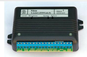
**Link Lift Watch provides communication** between a lift cabin and hotline service (first aid) via PSTN network. After pressing the alarm button on the control panel in the lift cabin the Link Lift Watch automatically dials up preprogrammed number (up to 6) and establishes connection with hotline service (first aid).
