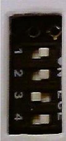
The program reads the DIP Switch state after restart. The DIP switch has 4 switches.
